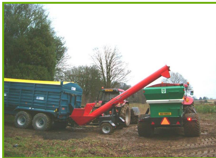
Picture 31. Sewage Sludge being elevated into the injection trailer. [Photo by: UFU]
