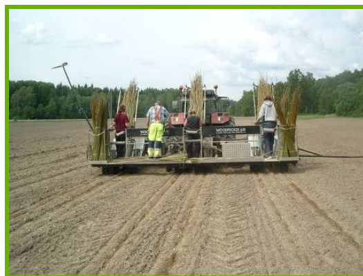
Picture 11. For SRP planting different types of machinery can be used. The time and work load required for one hectare of short cuttings planting (A) is much larger than for long rod step-planting (B). [Photos by: T. Tilger, EAU; N.-E. Nordh, SLU respectively]
