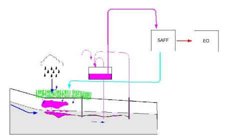
with Surface Active Foam Fractionation (saff) technology and the PFAS constituent destroyed by oxidation. It is estimated that this could reduce the treatment time by a factor of 10 to 20.
